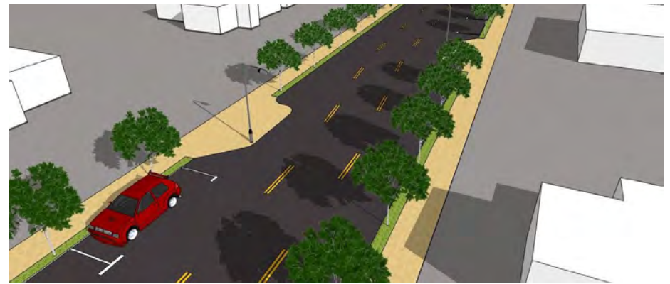
Figure 15: Illustration of design elements intended to reduce vehicle speed Introducing new design elements like trees, bulb-outs, pedestrian crossings, and even on-street parking can have the combined effect of reducing how fast drivers can comfortably operate and creating a safer and more attractive environment for other users and adjacent businesses and residents.
