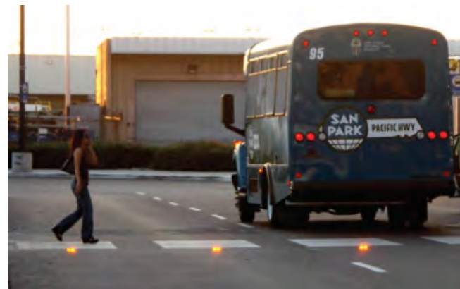
Figure 8: In-road lighting More reliable hardware for in-road lighting offers improved visibility in reversible lanes and crosswalks.
