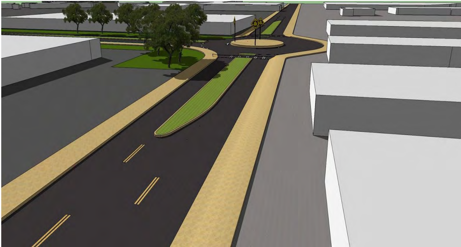
Figure 24: Illustration of proposed lane configuration and roundabout at BeltLine/ Bill Kennedy Way (aerial looking west)
