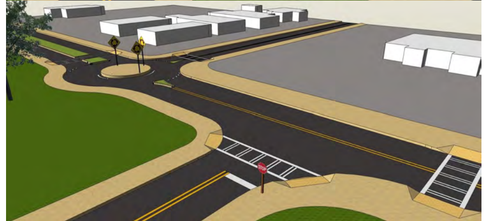
Figure 31: Illustration of roundabout at Whitefoord with elimination of signal at Memorial Terrace
