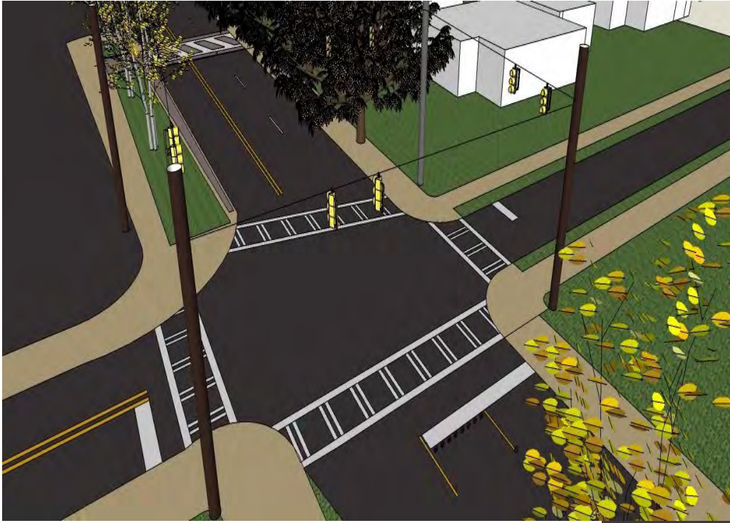
Figure 20: Illustration of proposed intersection redesign and lane reconfiguration at Clifton Street (aerial looking northwest)
